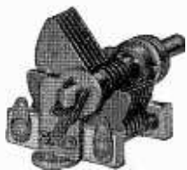
Single 0.00014 mfd. Hammarlund condenser; non-inductive pigtail; single hole panel mount and two-point base mount; Isolantite insulation; brass plates.
